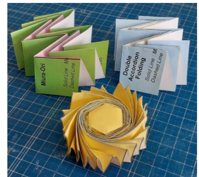
Fig.2 Origamis considering the paper thickness: Miura-Ori (Upper Left), Double Accordion Folding (Upper Right) and Spiral Folding (Lower Middle)
