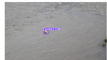
Automatic detection of PET bottles flowing in rivers using AI
